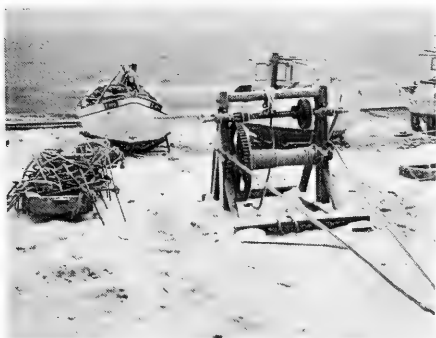
Beach landing craft used for inshore fishing in Denmark. Note portable roller used for beaching the boats.
